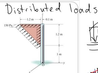
To be able to design the joint between the sign and the sign post, we need to determine a single equivalent resultant force and its location.
