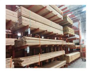
The lumber places a distributed load (due to the weight of the wood) on the beams. To analyze the load's effect on the steel beams, it is often helpful to reduce this distributed load to a single force. How would you do this?
