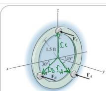
The three parallel bolting forces act on the circular plate, such that  $F_A = F_B = F_C = F > 0$ . Replace the force system by a resultant force  $F_R$  and a resultant moment  $(M_R)_0$  about the origin.
